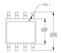
DIMENSIONS IN INCHES  $\frac{\text{MIN.}}{\text{MAX.}}$  LEAD COPLANARITY 0.004 MAX.
