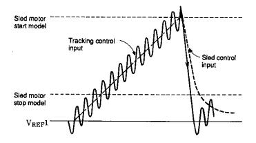
The start and stop levels are set by an external resistor connected between the V<sub>REF</sub>1 pin and the REFO pin.
