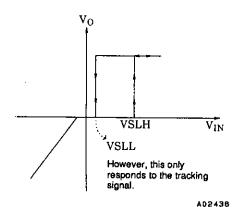
Note that for inputs that are lower than V<sub>REF</sub>1 this system operates normally regardless of the SLS pin.
