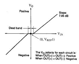
That is, the LB8107M implements a polarity reversing V-type drive with respect to the input signals (from the DSP) referenced to  $V_{REF}1$ .
