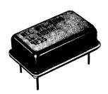
The common thread running through the NTC-4000 TCXO family is its use of our custom bipolar three segment compensation IC. In addition to the IC and the crystal, these oscillators have adjustable thick film resistors for compensation and varactors to provide the changing reactance for temperature compensation. The NTC-4000 Series is available in a hermetically sealed, leaded DIP.
