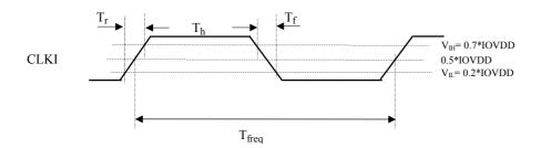
$\begin{array}{ll} Measurement \ point \\ V_{IH} &= 0.7*IOVDD \\ V_{IL} &= 0.2*IOVDD \\ V_{OH} &= 0.8*IOVDD \end{array}$
