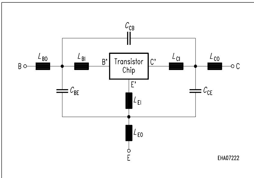
To avoid high complexity of the package equivalent circuit, both emitter leads of TSFP-4 are combined in one electrical connection.  $R_{LXI}$  are series resistors for the inductances  $L_{XI}$  and  $K_{xa-yb}$  are the coupling coefficients between the inductances  $L_{xa}$  and  $L_{yb}$ .
