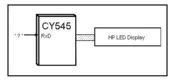
Each query command will output the current value of the requested parameter. For the user-bits query, a 16-bit value is returned, with the lower 8 bits corresponding to the CY545 User Bits, and the upper 8 bits corresponding the the CY545 Data bus.
