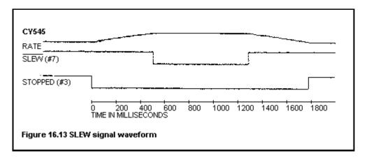
The SLEW signal may also be used as an input. If this signal is driven low before the beginning of a motion, the CY545 will enter the continuous stepping mode. In this mode, it will accelerate
