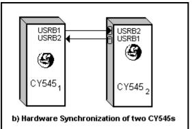
Note that when the two programs are not identical, the master can also use a Wait command, while the slave executes its own Bit instruction, to achieve a more general synchronization.
