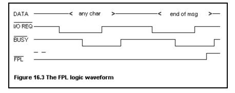
Notice that the FPL signal is removed at the end of the message, while the CY545B is still Busy, but after the I/O Request has been driven high again.
