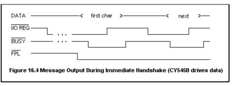
After the CY545B has issued the output message, and FPL is high again, the host may continue with the immediate command handshake, and the CY545B will now accept and execute the immediate command as shown in the second example waveform below. Here, the host does not drive the data bus for the first handshake, and thereby gives the CY545B the "OFFh" first command character prefix. This is followed by the normal first command character.
