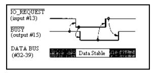
This function is repeated until all command characters have been issued to the CY545. In direct command mode, the CY545 executes every command as it is received. This means that the CY545 will go busy for a longer period of time with the last character of a command, while the command is actually executed. For long time delays or long motions, this time could be many seconds.
