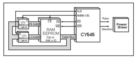
The CY545 provides all address and strobe timing signals to the memory. Signals involved are the data bus, XMEM\_SEL, ALE, WR, and RD. Special use is made of the data bus, which provides all 16 bits of address, plus the actual data transfers. Two external latches are required to hold the address. The example uses 74LS373s for this purpose.
