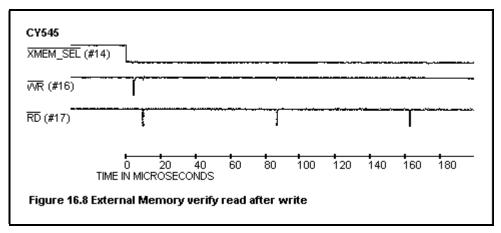
You should be aware of this time period delay when using EEPROM, because it is possible to send serial characters to the CY545 faster than the EEPROM can accept them, when running the serial interface at higher baud rates. It is best to have a time delay between each character in this case, or else use the CTS signal to hold off the communications until the CY545 is ready.
