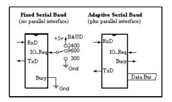
An alternative method of selecting the baud rate is through a parallel Mode command. For this command, nine baud rate selections are available, from 300 to 57600, plus the self adaptive rate. Details of the Mode command are described in a later section.
