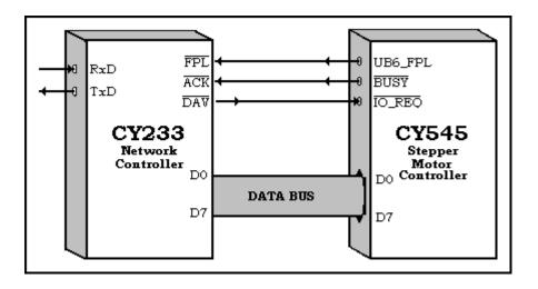
The CY233 Network Control chip allows you to connect up to 255 devices to a single RS-232 serial communications line such as an IBM-PC COM1 or COM2 port, with unique addresses assigned to each device. The CY233 Network is ideal for distributed systems where central control is required but very high speed communication is unnecessary.
