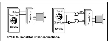
If the user opts for his own driver design, the PULSE and CCW lines may be used to drive a counter circuit, which counts up or down once for each pulse, based on the level of the CCW signal. The counter output then drives the address lines of a memory device, such as a PROM, EPROM, or EEPROM, with data outputs that generate the desired motor phase patterns as the counter address steps through the PROM locations. This design is shown here.
