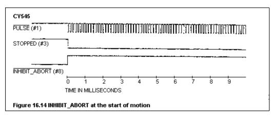
Once the motor is moving, the INHIBIT\_ABORT signal may be used to slow down and stop a motion before the CY545 reaches the target position. Using the signal in this way provides a controlled early stop to the motion.
