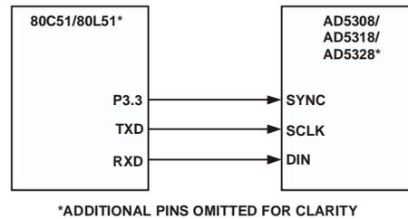
Figure 15. 80C51/80L51 to AD5308/AD5318/AD5328 Interface
