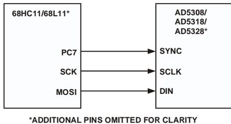
Figure 14. 68HC11/68L11 to AD5308/AD5318/AD5328 Interface
