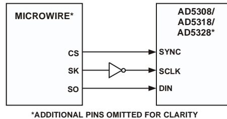
Figure 16. MICROWIRE to AD5308/AD5318/AD5328 Interface
