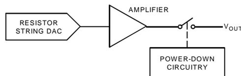
Figure 12. Output Stage During Power-Down
