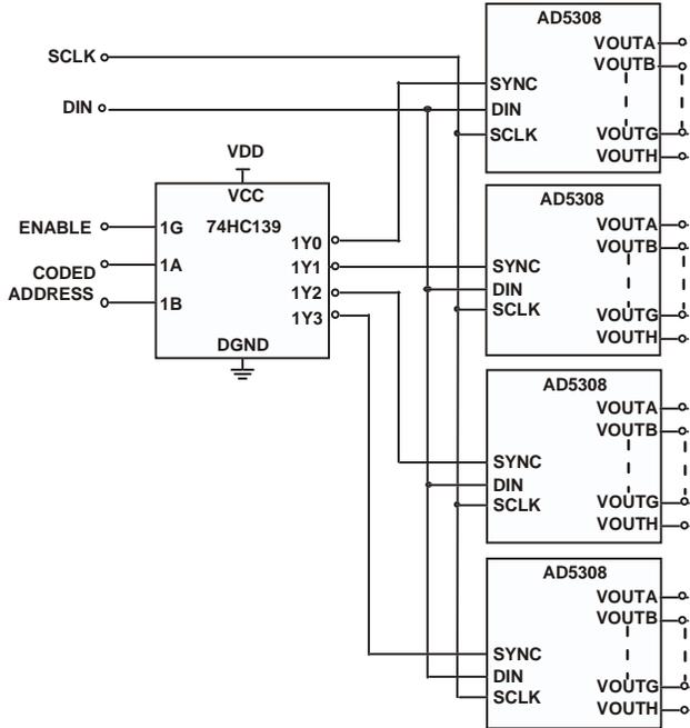
Figure 20. Decoding Multiple AD5308 Devices in a system
