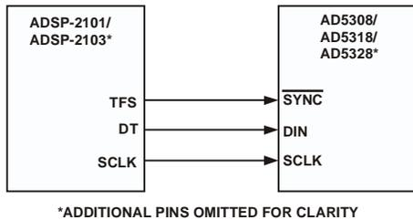
Figure 13. ADSP-2101/ADSP-2103 to AD5308/AD5318/AD5328 Interface
