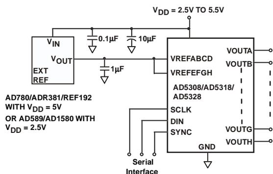
Figure 17. AD5308/AD5318/AD5328 Using a 2.5 V External Reference
