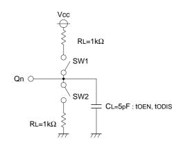
0 ~ 3V Input pulse level: Input pulse rise time and fall time: 3ns Measurement reference level, input: 1.3V
