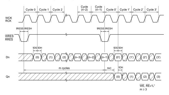
n-bit delay 2 (Sliding WRES and RRES at a cycle corresponding to delay length)
