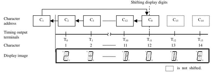
In this setting, the display images of "2", "3", - - appear on the  $T_0$ ,  $T_1$ ,  $T_2$ , - -  $T_{10}$  pins respectively, and the image "0" is on the  $T_{11}$  pin, which is assigned to the 12<sup>th</sup> character address. The display images "D" and "E" don't shift but remain on the  $T_{12}$  and  $T_{13}$  pins, assigned to the 13<sup>th</sup> and 14<sup>th</sup> characters respectively, because their character addresses are outside the digit "N".
