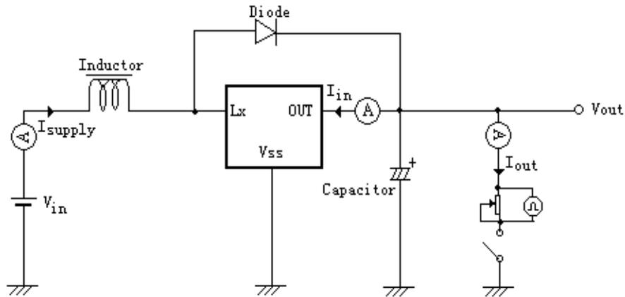
Inductor:  $47 \mu\text{H}$ ; Diode: 肖特基二极管(正向压降约  $0.2\text{V}$ );
