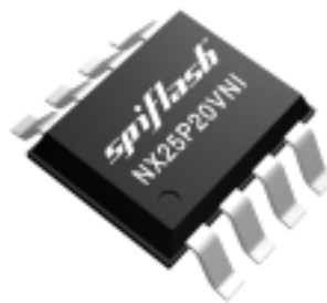
8-Pin SOIC 150-mil (Package Code N)
