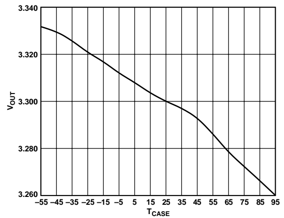
Figure 6. Output Voltage vs. Case Temperature (°C) (ADDC02803SC)
