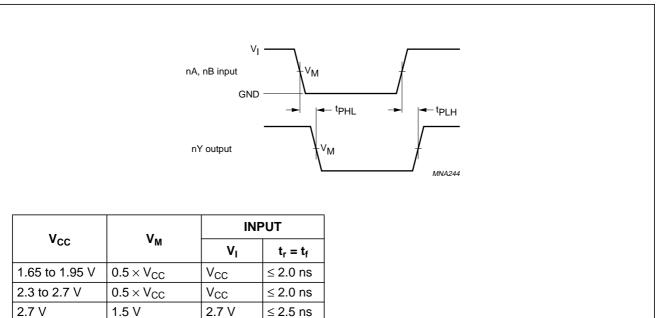
Fig.5 Inputs nA, nB to output nY propagation delay times.
