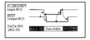
This function is repeated until all command characters have been issued to the CY545. In direct command mode, the CY545 executes every command as it is received. This means that the CY545 will go busy for a longer period of time with the last character of a command, while the command is actually executed. For long time delays or long motions, this time could be many seconds.
