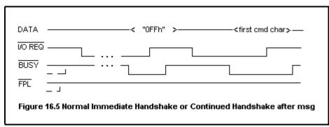
Also note that the second example waveform applies to the case where the CY545B accepts the immediate command without first generating some output data.
