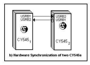
Note that when the two programs are not identical, the master can also use a Wait command, while the slave executes its own Bit instruction, to achieve a more general synchronization.
