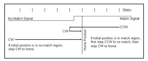
If the home sensor signal cannot be designed to indicate the initial direction to home, the motor must be positioned so that it is on the "correct" side of home before the Home command is used. This will insure that the CY545 always steps towards the sensor on seeking the home position. The CW and CCW limits might be useful in this situation, since you could move to a known limit, then use the home command to step in the opposite direction until the home position is found.
