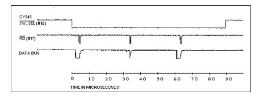
To read an entire parameter, the digit read process is repeated three, five, or eight times, depending on the size of the parameter. The CY545 starts by reading the most significant digit, then the next, until it finally reads the least significant digit. This is the same order that digits are read from a command with numeric arguments.
