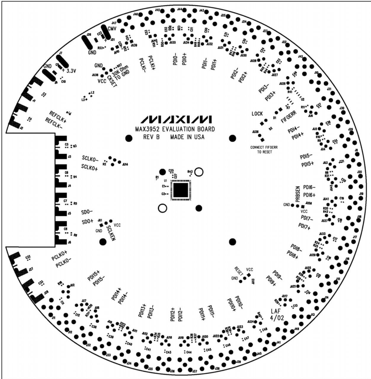
Figure 4. MAX3952 EV Kit Placement Guide—Component Side
