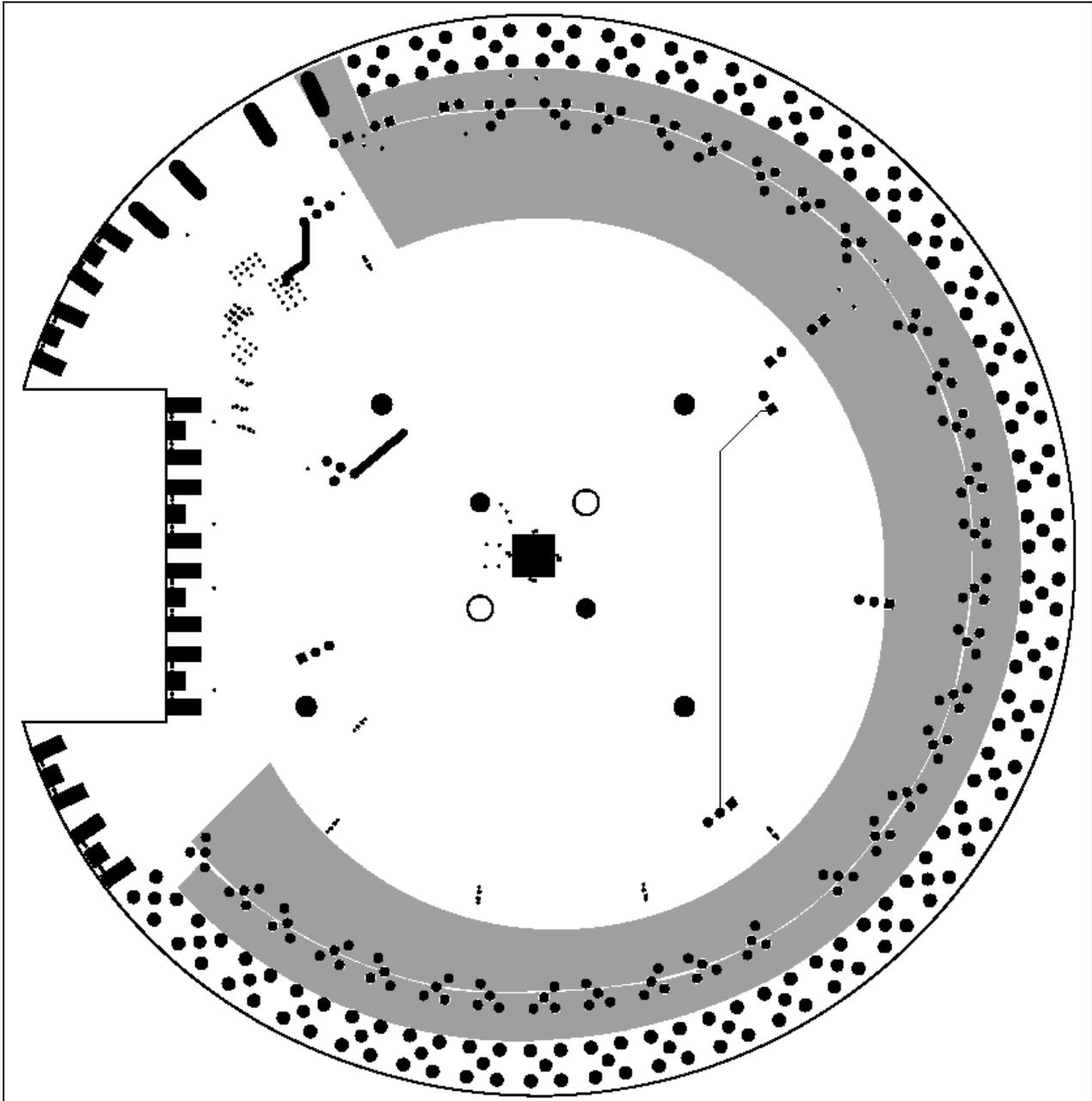
Figure 5. MAX3952 EV Kit Component Placement Guide—Solder Side
