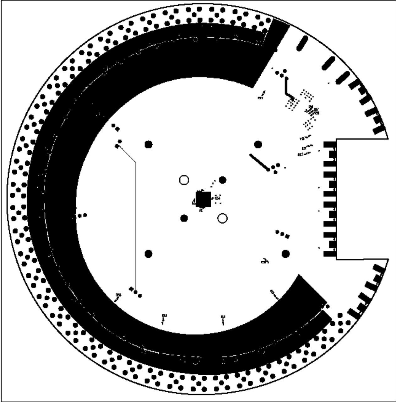
Figure 6. MAX3952 EV Kit PC Board Layout—Solder Side
