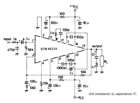
Sample Application Circuit (40W min AF Power Amplifier)
