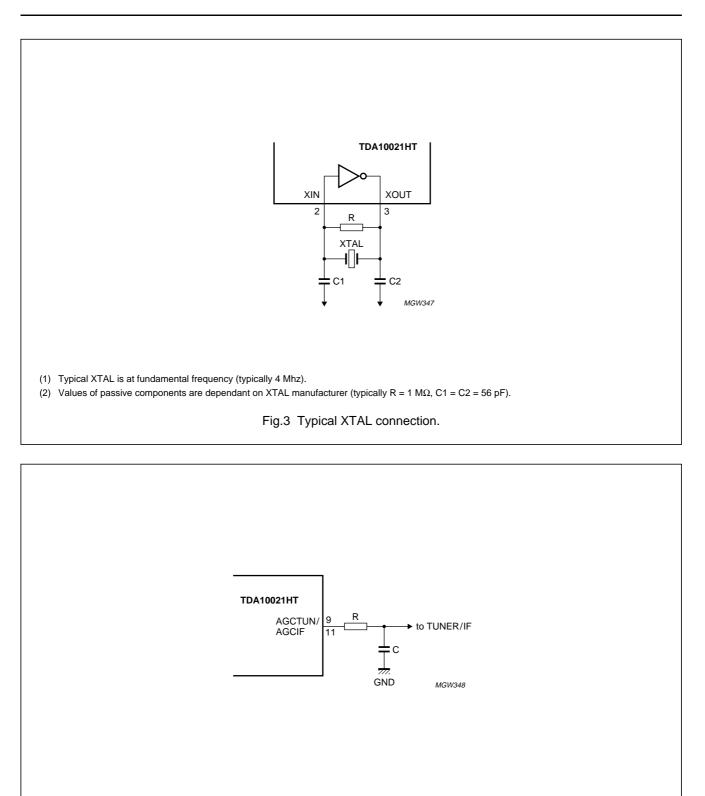
R and C are chosen to verify  $\frac{SR}{1024}$  <  $f_c < \frac{XIN}{16}$  with R = 1.5 k $\Omega$  and C = 1 nF,  $f_c$  = 100 kHz.
