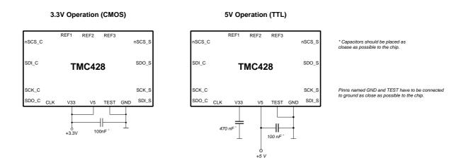
Figure 19 - 3.3V Operation (CMOS) vs. 5V Operation (TTL)
