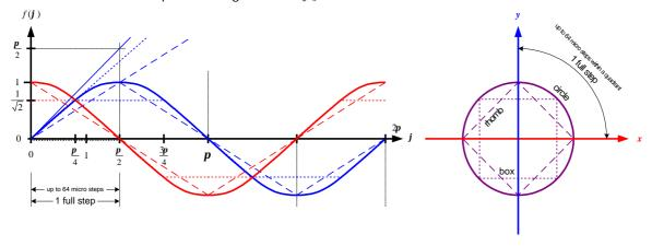
Figure 16 - micro step enhancement by introduction of a shape function  $f_s(\mathbf{i})$
