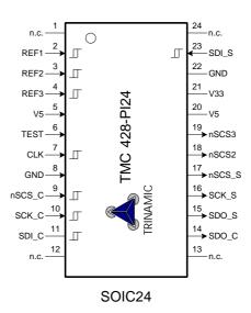
Figure 3: TMC428 pin out
