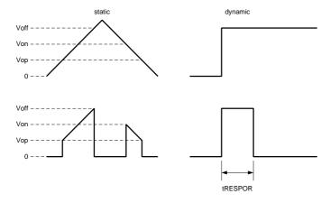
Figure 21 - Operating Principle of the power-on-reset
