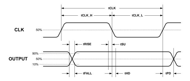
Figure 20 - General Timing Parameters
