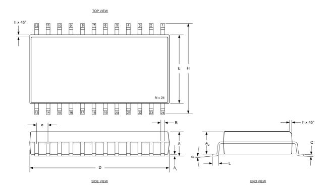
Figure 18 - Package Outline Drawing SOIC24, 300 MILS
