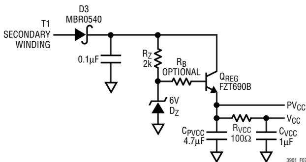
Figure 8.  $V_{CC}/PV_{CC}$  Regulator
