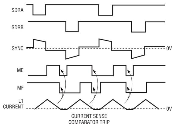
Figure 6a. Discontinuous Mode Operation at No Load
