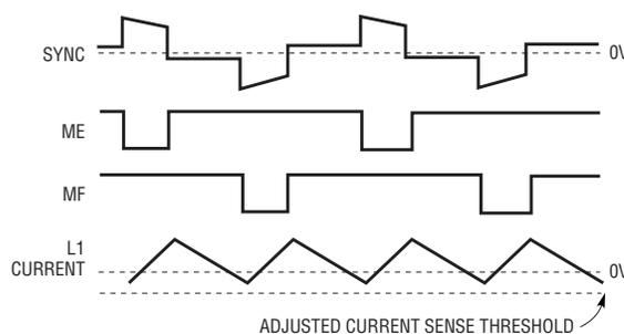
Figure 6b. Continuous Mode Operation with Adjusted Current Sense Threshold
