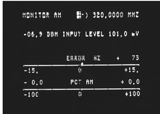
Figure 29. Power Output of Unmodulated Carrier
