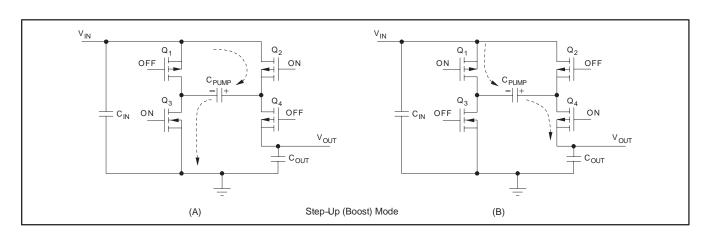
Figure 2. Simplified Schematic of the REG710 Operating in the Step-Up or Boost Mode
