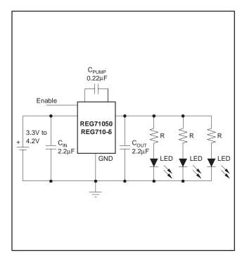
Figure 7. REG710 Circuit for Driving LEDs
