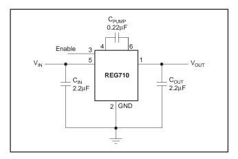
Figure 3. Typical Operating Circuit
