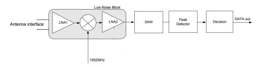
Figure 11: Receiving Link Block Diagram
