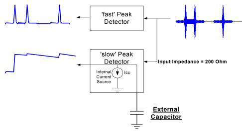
Figure 13: Peak Detectors & ASK Receiver
