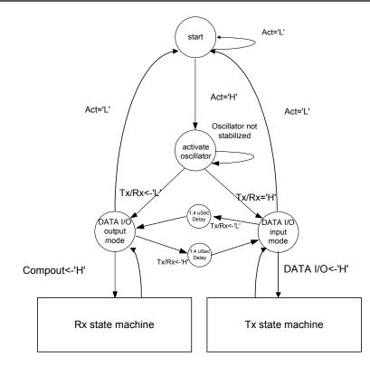
Figure 15: General State Machine Block Diagram
