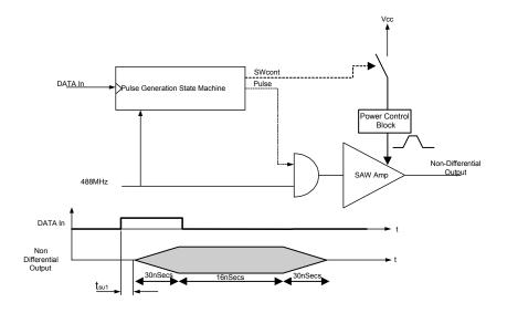
Figure 9: Pulse Generator Block Diagram
