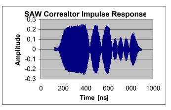
Figure 5: Pulse Response of the Correlator - Measured
