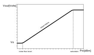
Figure 12: Peak Detector Vout (Pin) Graph
