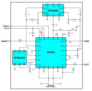
Figure 2: Transceiver Implementation - Using RFW102 Chipset
