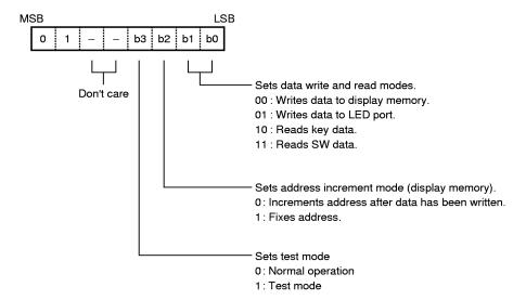
On power application, the normal operation mode and address increment mode are set.
