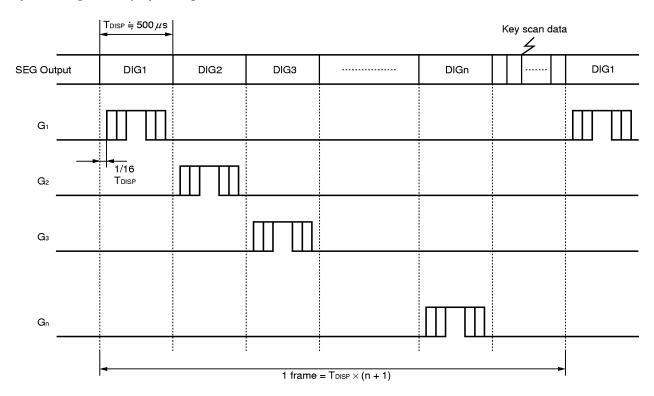
One cycle of key scanning consists of two frames, and data of  $12 \times 4$  matrices is stored in RAM.
