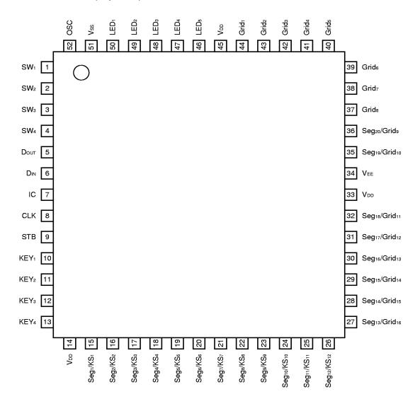
Use all the power pins. Leave the IC pin open.
