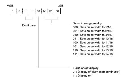
On power application, the 1/16-pulse width is set and the display is turned off.
