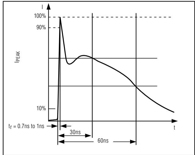
Figure 8. IEC 1000-4-2 ESD Generator Current Waveform
