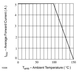
Figure 1. Max. Average Forward Current vs.
