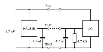
Fig. 4-1: Recommended application circuit
