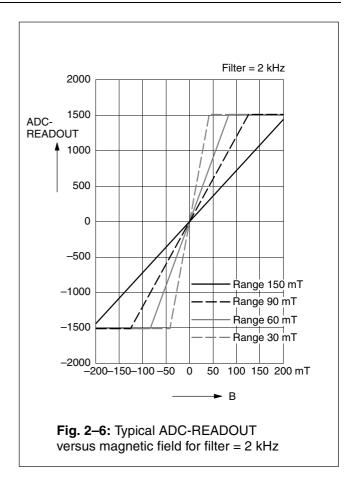
During further processing, the digital signal is multiplied with the sensitivity factor, added to the quiescent output voltage and limited according to the clamping voltage. The result is converted to an analog signal and stabilized by a push-pull output transistor stage.
