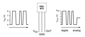
Fig. 2-1: Programming with V<sub>DD</sub> modulation
