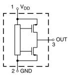
Fig. 1–1: Pin configuration
