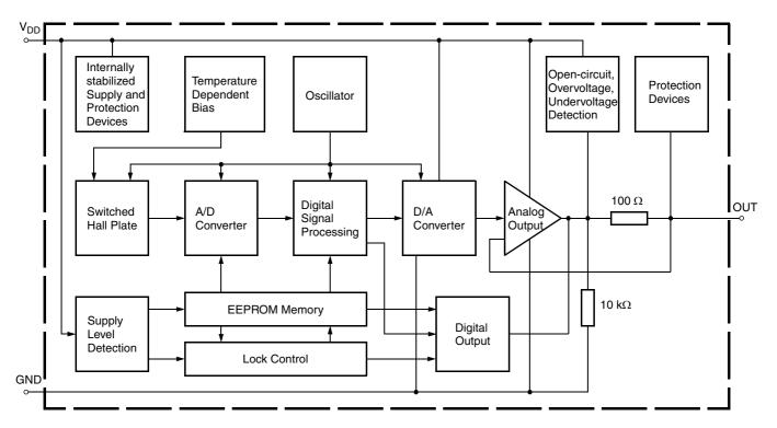
Fig. 2-2: HAL815 block diagram
