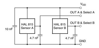
Fig. 4-2: Parallel operation of two HAL815
