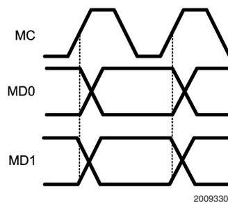
FIGURE 8. Dual Link Timing (READ)
