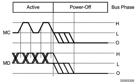
FIGURE 10. Bus Power Down Timing
