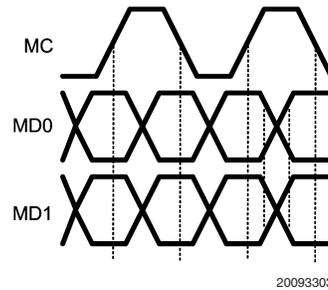
FIGURE 7. Dual Link Timing (WRITE)
