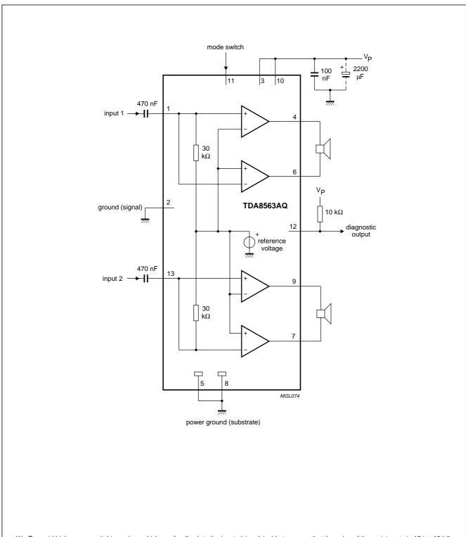
(1) To avoid high energy switching pulses which can feedback to the inputs it is advisable to ensure that the value of the resistor at pin 12 is  $\geq$ 10 k $\Omega$ .
