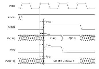
Figure 34. Channel mode interleaved format.
