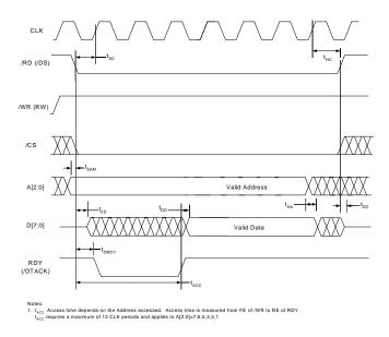
Figure 18. INM Microport Read Timing Requirements.
