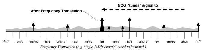
Figure 2a. AD6634 Frequency Translation of Wideband Input Spectrum
