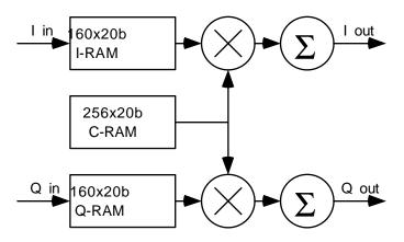
Figure 29. RAM Coefficient Filter Block Diagram
