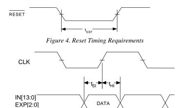
Figure 5. Input Data Timing Requirements
