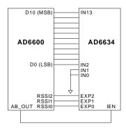
Figure 27. Typical Interconnection of the AD6600 gainranging ADC and the AD6634.
