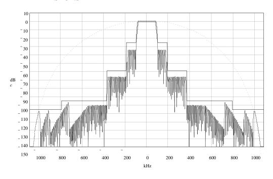
Figure 21. The filter above is based on a 65 MSPS input data rate and an output rate of 541.6666 kSPS (2 samples per symbol for EDGE). Total decimation rate is 120 distributed between the rCIC2, CIC5 and RCF.
