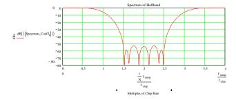
Figure 30. Interpolating Halfband Frequency Response
