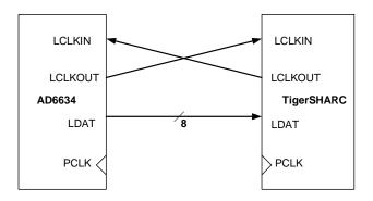
Figure 38. Link Port Connection Between AD6634 and TigerSHARC
