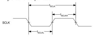
Figure 42. SCLK Timing Requirements
