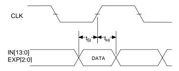
Figure 23. Input Data Timing Requirements
