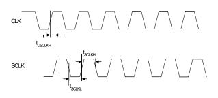
Figure 43. SCLK Switching Characteristics (Divide by 1)
