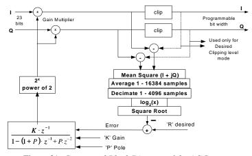
Figure 31: Conceptual Block Diagram of the AGC
