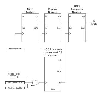
Figure 32. NCO Shadow Register and Hold Off Counter
