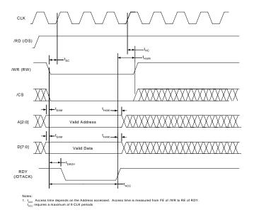
Figure 17. INM Microport Write Timing Requirements.
