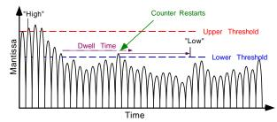
Figure 25. Threshold Settings for LI
