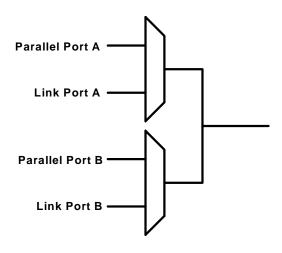
Figure 33 Output port data routing.
