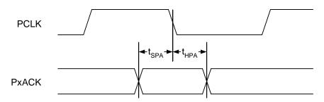
Figure 12. PxACK to PCLK Setup and Hold Characteristics
