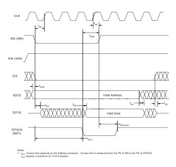
Figure 20. MNM Microport Read Timing Requirements.
