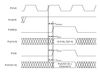
Figure 35. Channel mode 8I/8Q parallel format.
