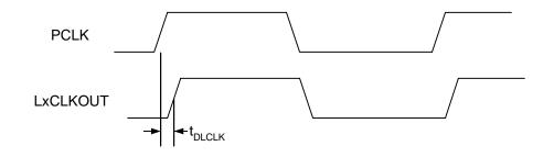
Figure 15. LxCLKOUT to PCLK Switching Characteristics
