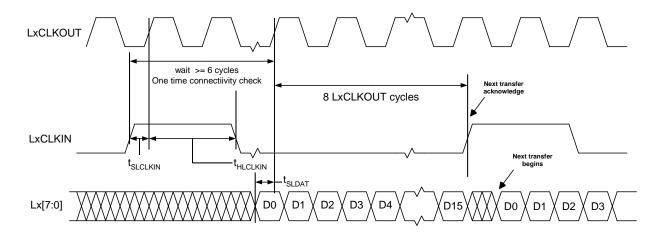
Figure 16. LxCLKIN to Lx[7:0]Data Switching Characteristics
