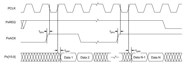
Figure 13. PxACK to PCLK Switching Characteristics
