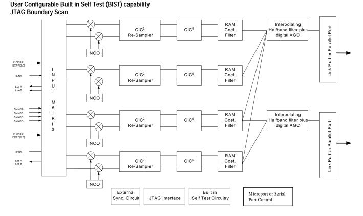
Figure 1. AD6634 Block Diagram
