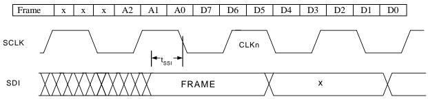
Figure 45. Serial Port Control Timing
