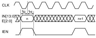
Figure 28. Fractional Rate Input Timing (4X CLK) in mode 01.
