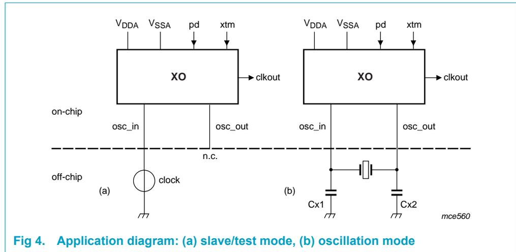
**Fig 4. Application diagram: (a) slave/test mode, (b) oscillation mode**
