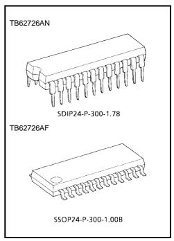
Weight SDIP24-P-300-1.78: 1.22 g (Typ.) SSOP24-P-300-1.00B: 0.32 g (Typ.)
