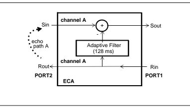
Figure 8 - Extended Delay Configuration (128ms)
