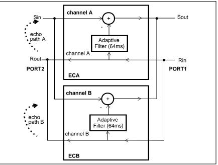
Figure 6 - Normal Device Configuration (64ms)
