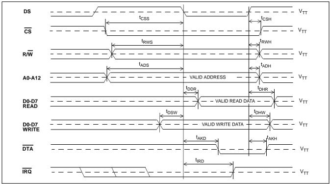
Figure 15 - Motorola Non-Multiplexed Bus Timing
