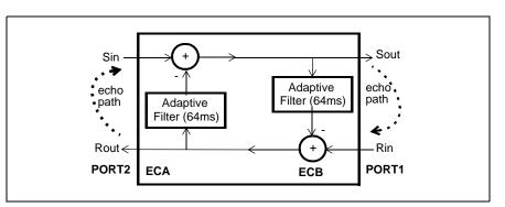
Figure 7 - Back-to-Back Device Configuration (64ms)
