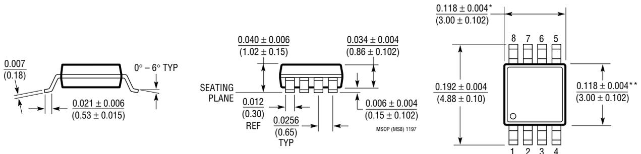
\* DIMENSION DOES NOT INCLUDE MOLD FLASH, PROTRUSIONS OR GATE BURRS. MOLD FLASH, PROTRUSIONS OR GATE BURRS SHALL NOT EXCEED 0.006\* (0.152mm) PER SIDE
