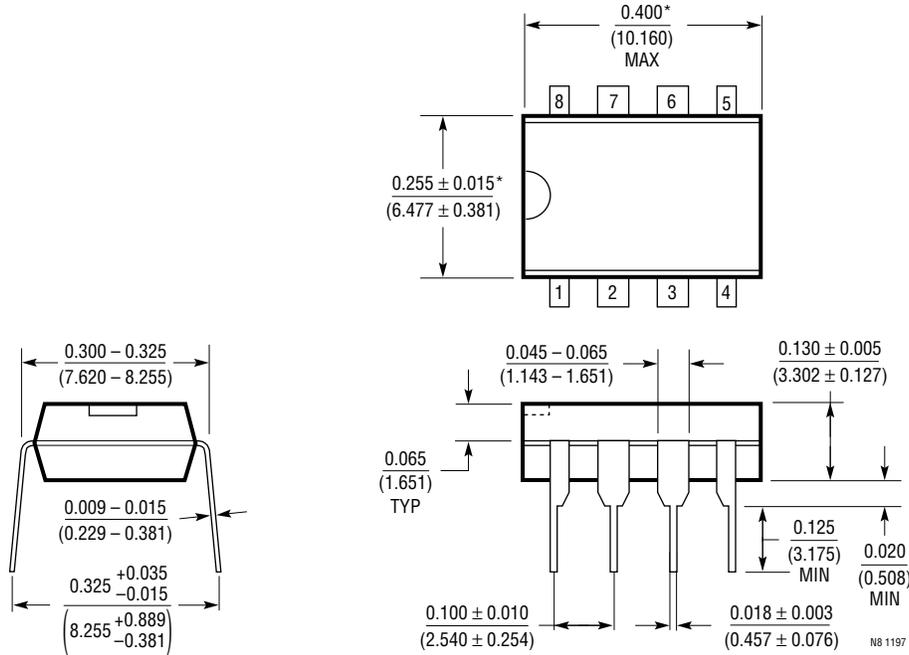
\*THESE DIMENSIONS DO NOT INCLUDE MOLD FLASH OR PROTRUSIONS.
