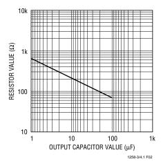
Figure 2. Damping Resistance vs Output Capacitor Value
