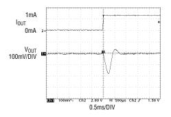
Figure 1. Reference Output Load Transient Response
