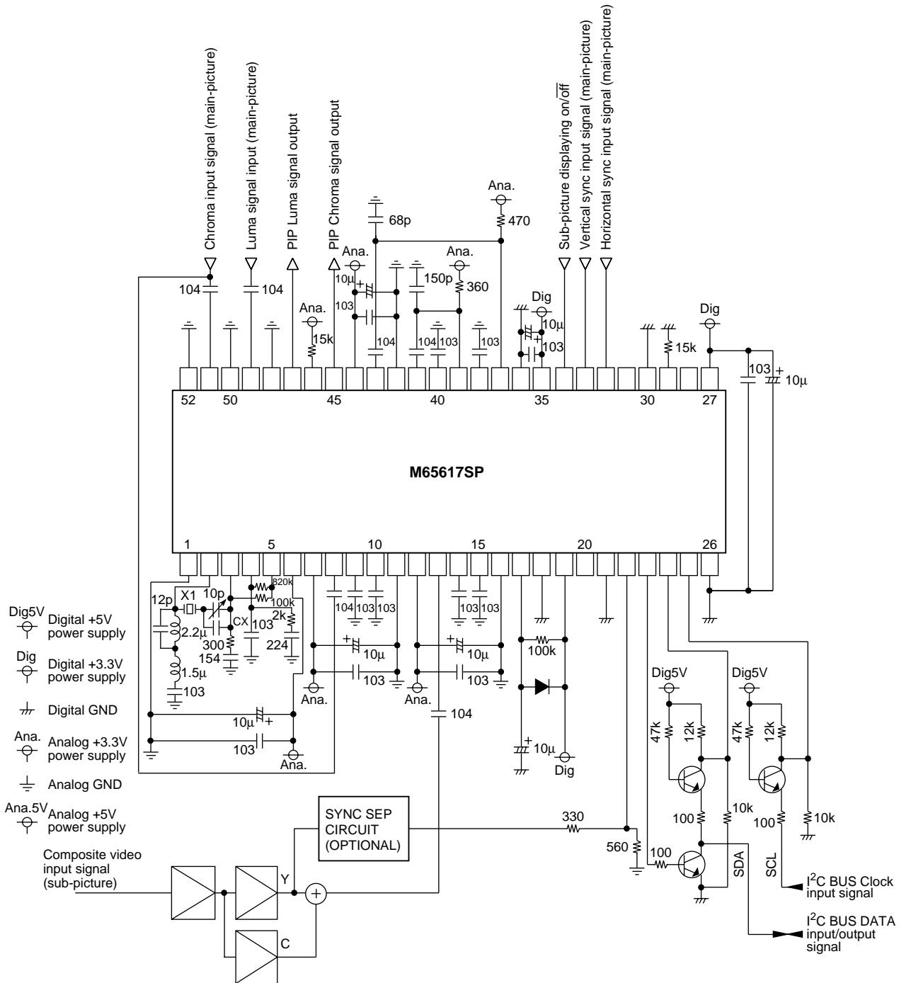
Separate Y/C signals by using LC-tank circuit or LPF,BPF for Y/C signals level adjust.
