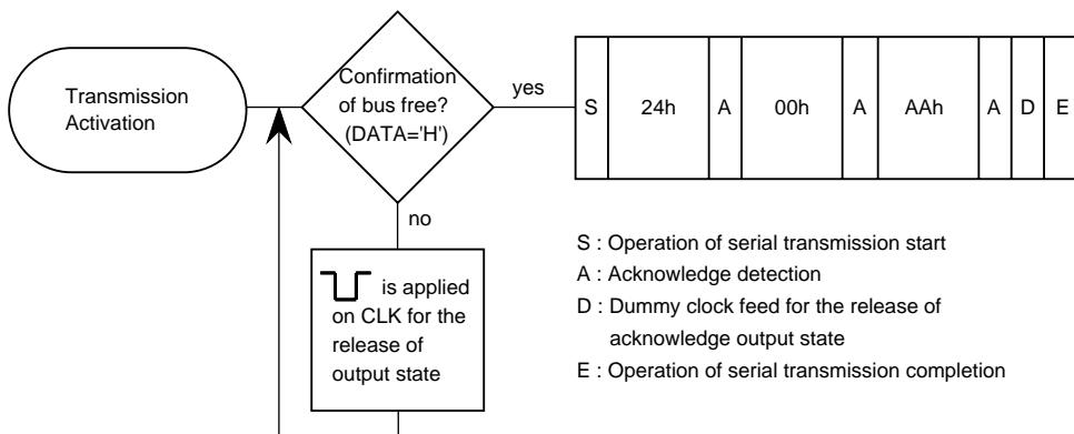
(2) Reading setting data FFh, 80h and EEh, individually, into internal address 04h to 06h of M65617SP:
