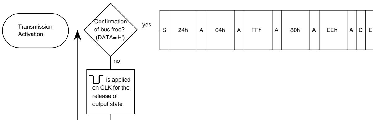
(3) Writing data on internal address 00h of M65617SP [Standard reading sequence version: 46 pin "L"]:
