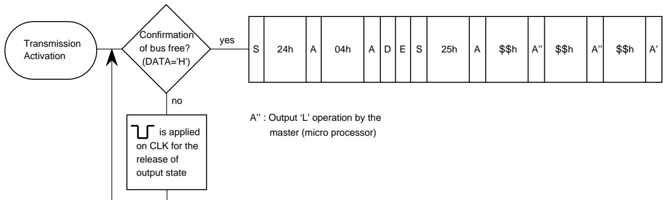
(5) Writing data on internal address 00h of M65617SP [Expanded reading sequence version: 46 pin " H "]:
