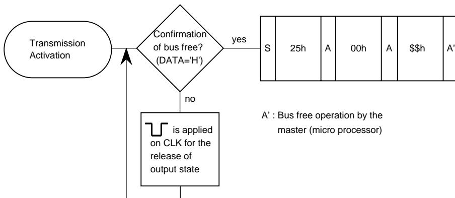
(6) Writing data on the internal address 04h to 06h of M65617SP [Expanded reading sequence version: 46 pin " H "]:
