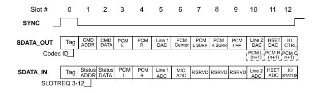
Figure 30. Standard Bi-Directional Audio Frame
