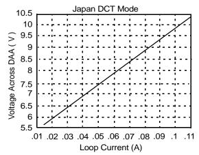
Figure 21. Japan Mode I/V Characteristics
