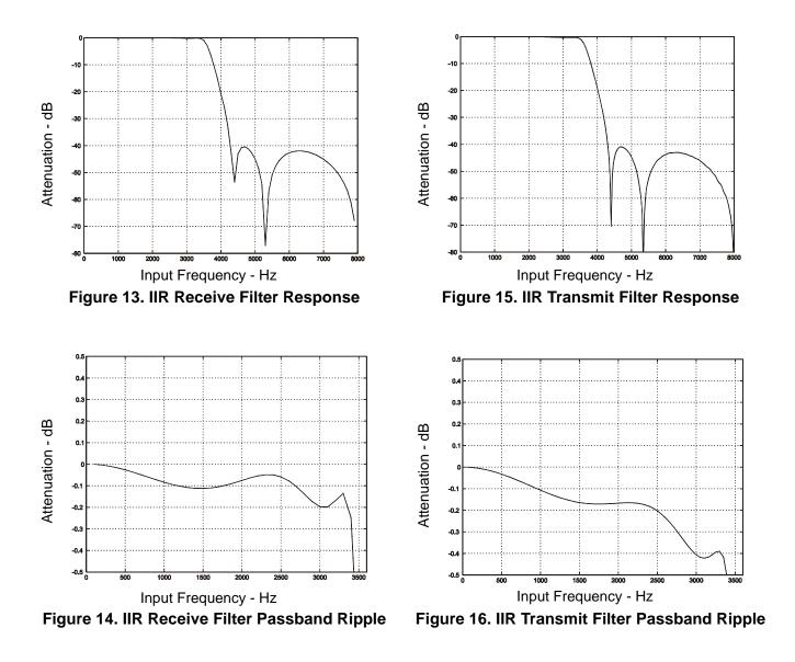
For Figures 13–16, all filter plots apply to a sample rate of Fs = 8 kHz. The filters scale with the sample rate as follows:
