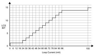
Figure 28. Typical LCS Transfer Function
