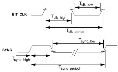
Figure 4. Clocks Timing Diagram
