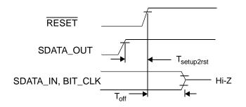
Figure 8. ATE Test Mode Timing Diagram
