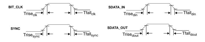
Figure 6. Signal Rise and Fall Timing Diagram
