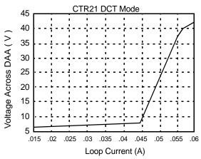
Figure 23. CTR21 Mode I/V Characteristics
