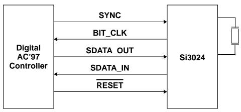
Figure 29. Si3038 Connection To AC'97 Controller (Primary Device Configuration)
