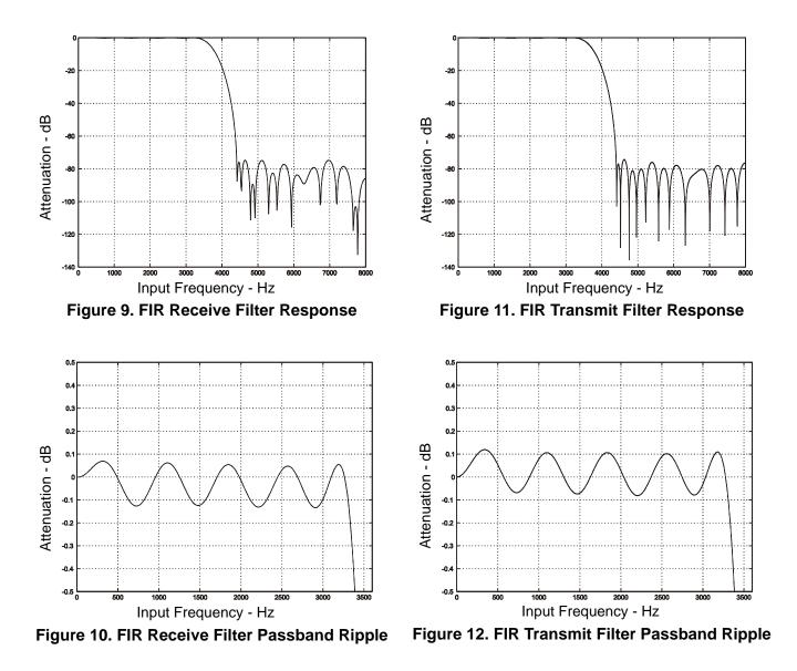
For Figures 9–12, all filter plots apply to a sample rate of Fs = 8 kHz. The filters scale with the sample rate as follows:
