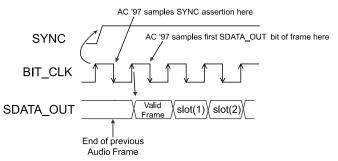
Figure 32. Start of an Audio Output Frame
