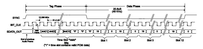
Figure 31. AC-Link Audio Output Frame
