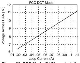
Figure 22. FCC Mode I/V Characteristics
