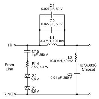
Figure 27. Dongle Applications Circuit
