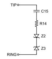
Figure 24. Ringer Impedance Network
