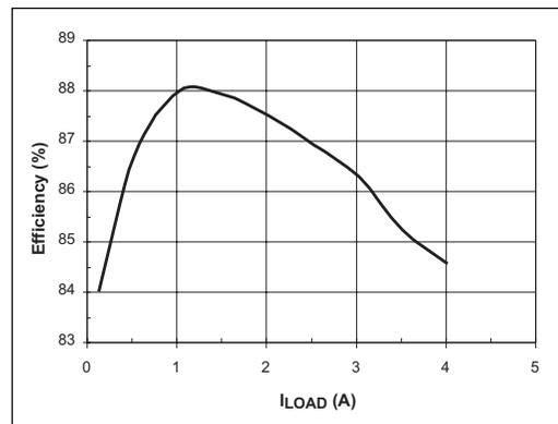
Figure 2. SP6122 Efficiency with  $V_{IN} = 3.3V$ ,  $V_{OUT} = 1.9V$ .
