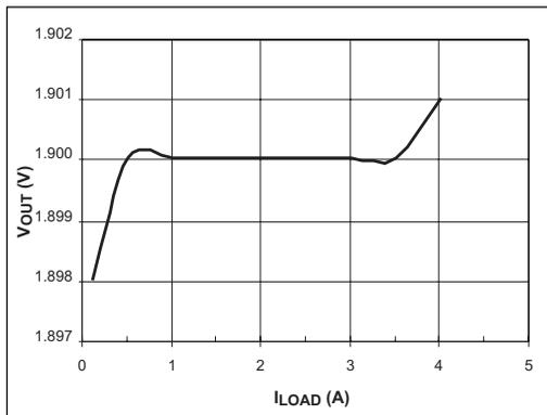
Figure 3. SP6122 Load Regulation with Input Voltage = 3.3V.
