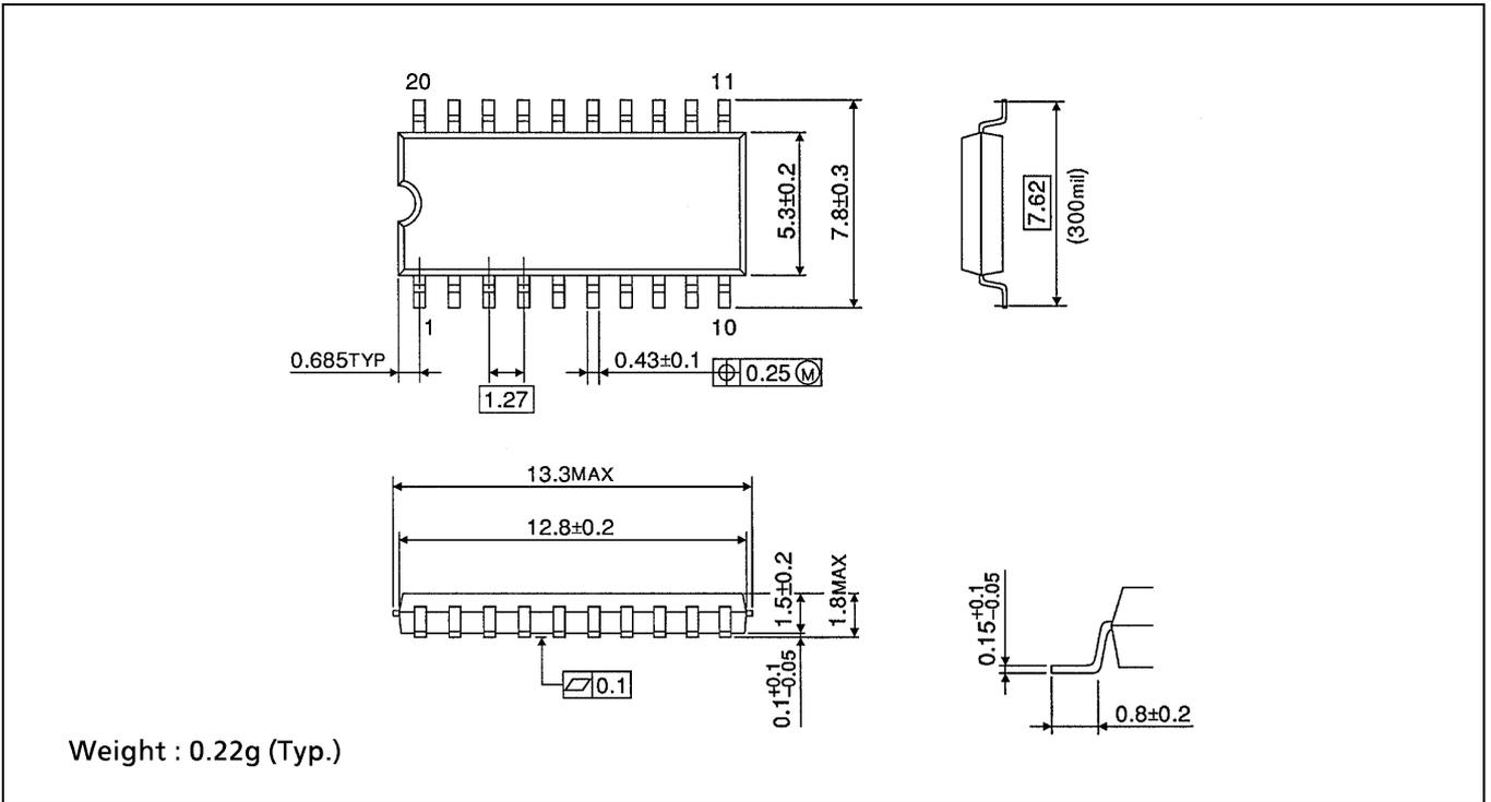
**SOP 20PIN (300mil BODY) PACKAGE DIMENSIONS (SOL20-P-300-1.27)**
