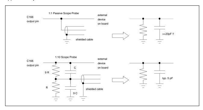
Different scope probes connected to signal lines influences the dynamic load of line drivers.
