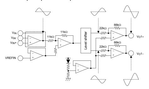
Note \*: Only channel 1 has an added input operational amplifier.
