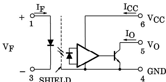
Note. A  $0.1\mu\text{F}$  bypass capacitor must be connected between pins 4 and 6.
