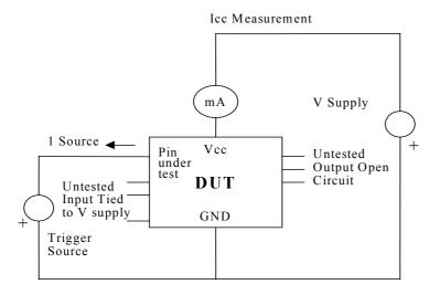
Test Circuit: Negative Input/ Output Overvoltage /Overcurrent
