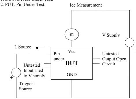
Test Circuit: Positive Input/ output Overvoltage/Overcurrent
