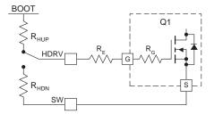
Figure 5. Driver dissipation model
