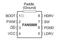
FAN5009MP 8-pin MLP package (Paddle should be connected to ground or left floating)
