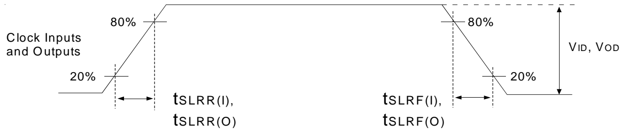
Figure 8. Input and Output Slew Rates
