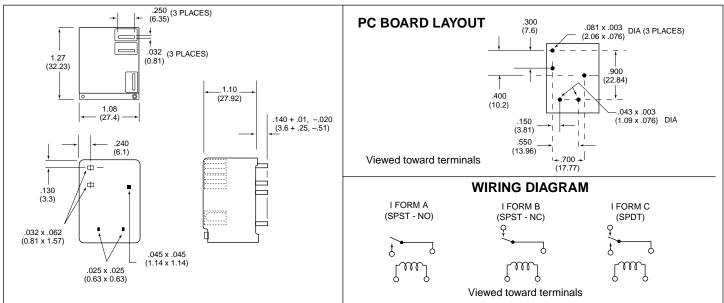
Dimensions in inches with metric equivalents in parentheses. Tolerance: ± .010"
