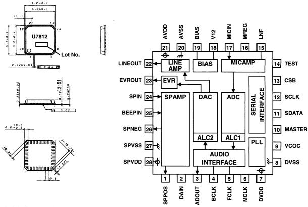
Note) Mounting on the portions indicated by dotted lines is not recommended.
