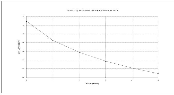
Figure 4 - AGCOUT characteristic versus AGCBIAS resistor
