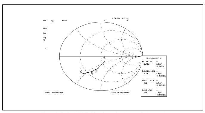
Figure 5 - Typical SAWF driver input impedance, single-ended
