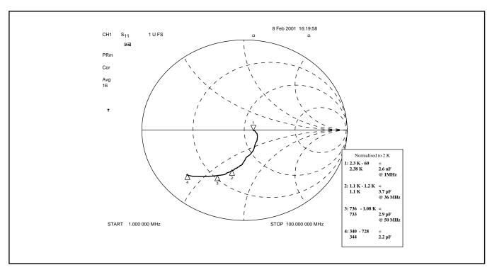
Figure 8 - Typical IF amplifier input impedance, single-ended
