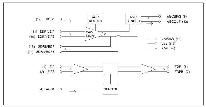
Figure 2 - Block diagram
