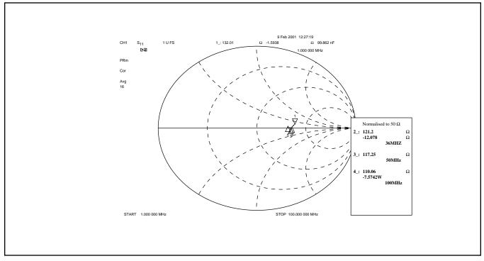
Figure 6 - Typical SAWF driver output impedance, single-ended
