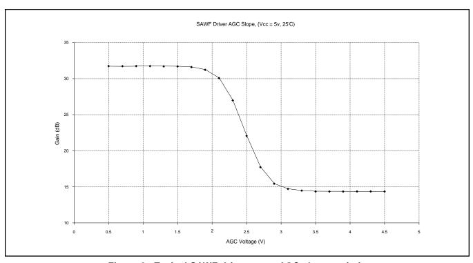
Figure 3 - Typical SAWF driver stage AGC characteristic
