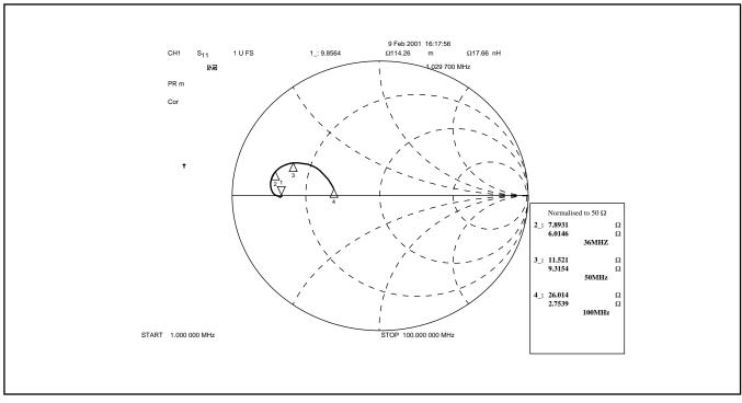
Figure 9 - Typical IF amplifier output impedance, single-ended
