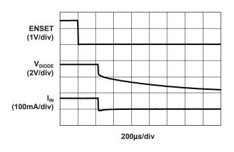
Load Switch to Charge Pump (80mA)
