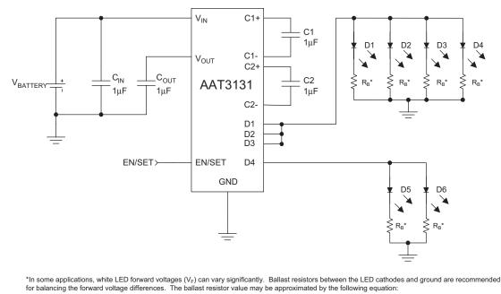
$R_{B} = \frac{V_{SOURCE} - V_{F}}{I_{E}}$
