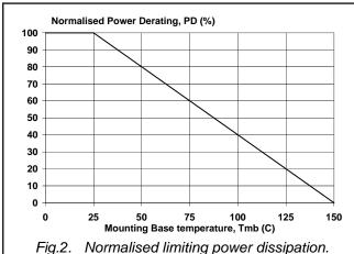
Normalised limiting power dissipation.  $P_D$ % = 100· $P_D$ / $P_D$ (25°C) =  $f(T_{mb})$
