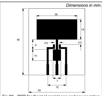
Fig.22. PCB for thermal resistance and power rating. PCB: FR4 epoxy glass (1.6 mm thick), copper laminate (35 μm thick).
