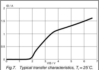
Fig.7. Typical transfer characteristics,  $T_j = 25$  °C.  $I_D = f(V_{IS})$ ; conditions:  $V_{DS} = 10$  V,  $t_p = 300$  µs
