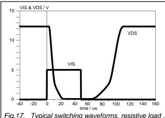
Fig.17. Typical switching waveforms, resistive load .  $R_L = 50 \Omega$ ; adjust  $V_{DD}$  to obtain  $I_D = 250$  mA;  $T_j = 25^{\circ}$ C
