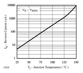
Figure 2. Reverse Current vs. Junction Temperature
