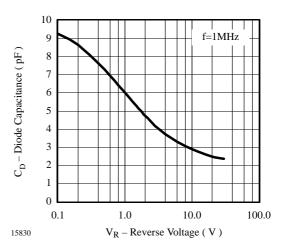
Figure 4. Diode Capacitance vs. Reverse Voltage
